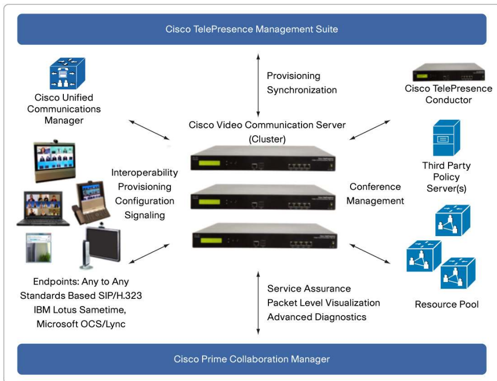
Figure 3. Cisco VCS Control in the Network
